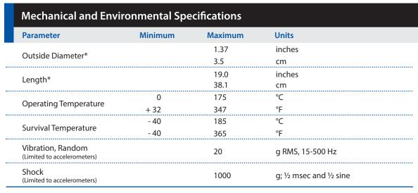
$<sup>\</sup>hbox{$^*$ Dimensions do not include running gear, centralizers, or axial shock absorbers.}$
