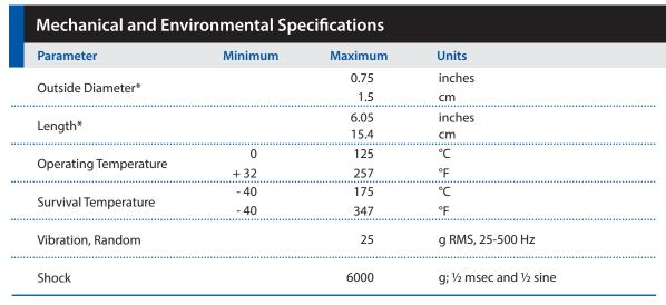
$<sup>\</sup>hbox{$^*$ Dimensions do not include running gear, centralizers, or axial shock absorbers}$
